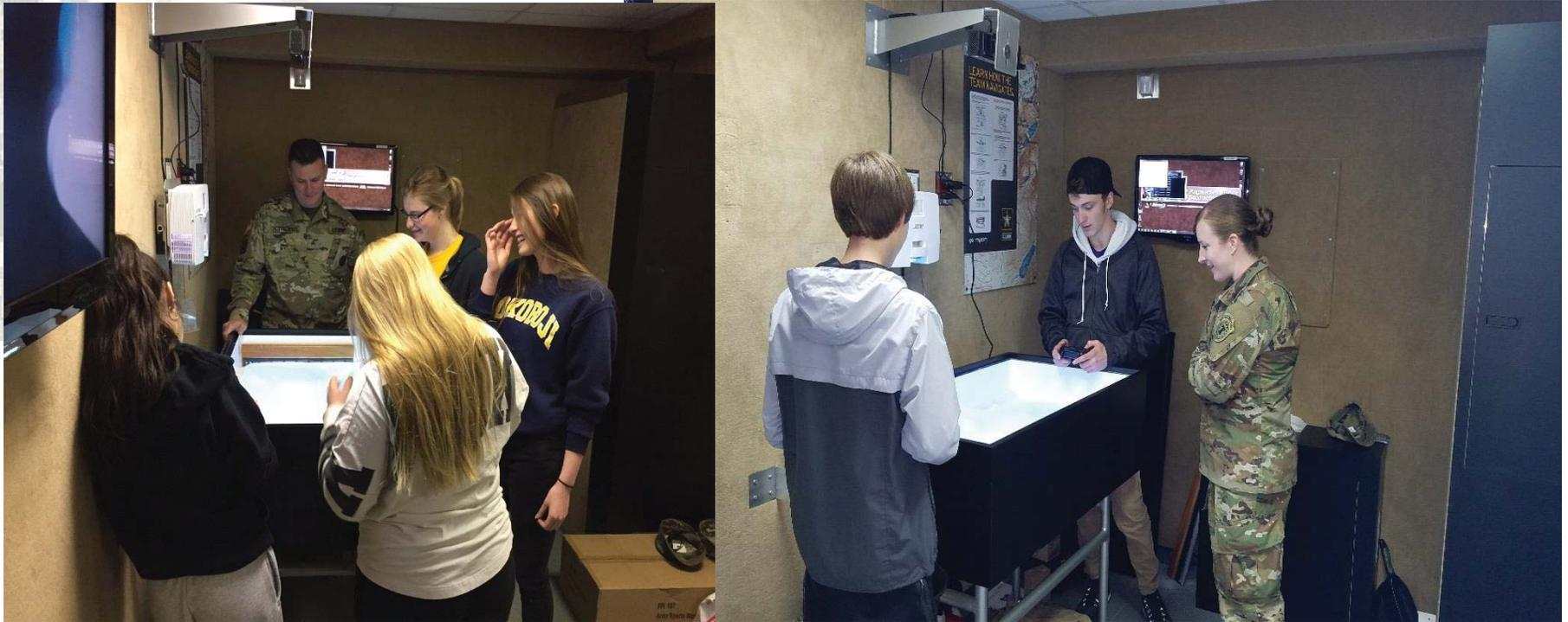
The Augmented Reality Sand table (ARES) is a traditional sand table, filled with play sand, augmented with a commercial-off-the-shelf projector, LCD monitor, laptop, and Microsoft Kinect. The Kinect senses user gestures, changes to the sand “terrain,” and potentially, verbal commands as forms of user interaction. ARES projects moving military units, terrain features, and other data onto the sand.
